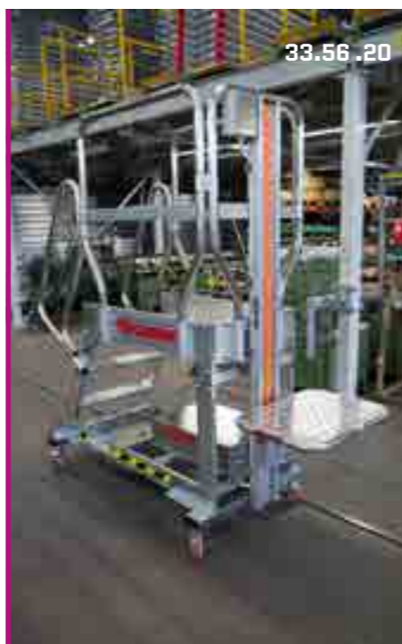
Scala a castello con piano picking elettrico. Bunk ladder with electric picking plane.
